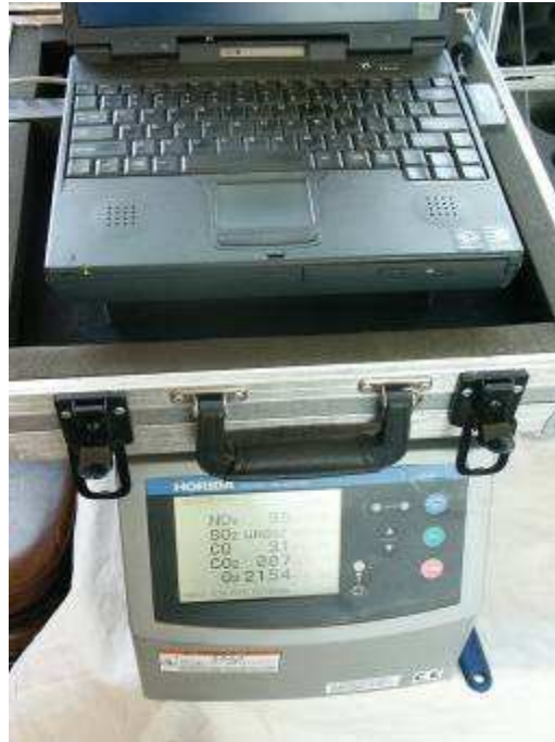
Figure 7-3 In-Field Illustration of Continuous Gas Analyzer and Computer for Data Logging
