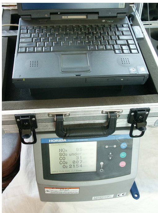
Figure A-0-3 In-field Illustration of Continuous Gas Analyzer and Computer for Data Logging
