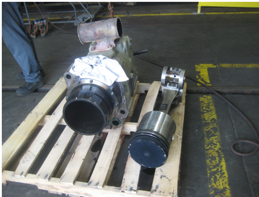
Figure 1. 2R Power assembly cylinder with piston removed
