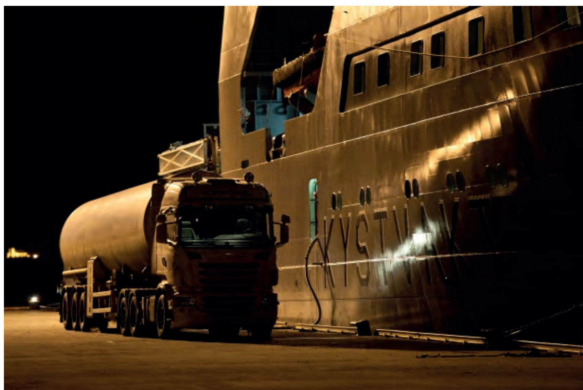
Figure 48: Truck to ship bunkering (TTS) of LNG
