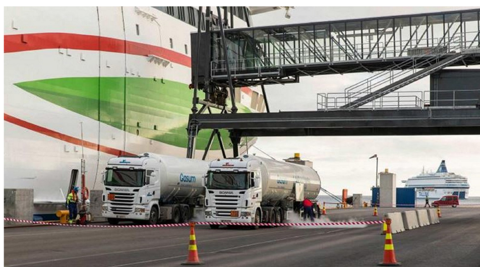
Figure 7. Truck-to-ship bunkering in the Port of Helsinki.
