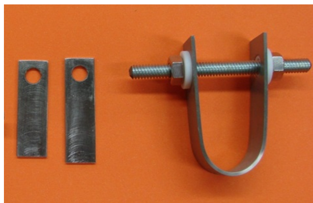
Figure 17. Photograph showing specimen geometries; unstressed alloy coupons (left two) and the U-bend sample (right). The distance of each end in the U-bend sample was approximately 2.5 cm (1 in.).
