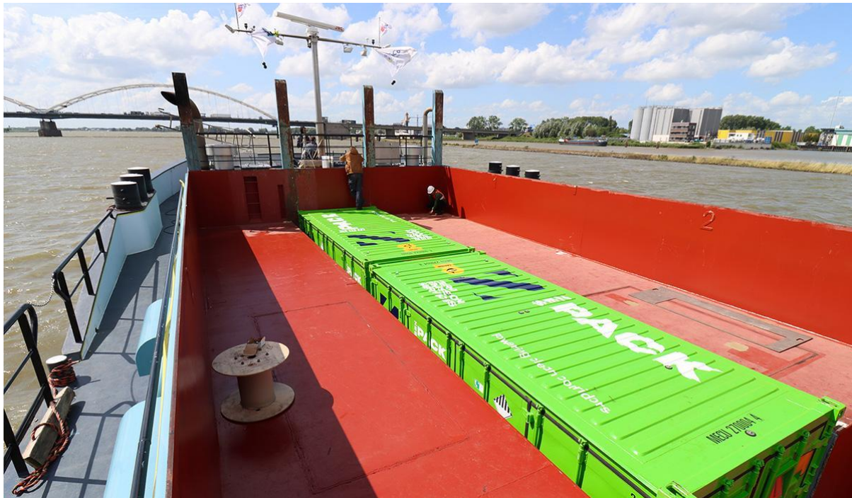
Figure 6: Swappable ESS in 20-foot ISO container operational on inland vessel Alphenaar (image: Zero Emission Services).
