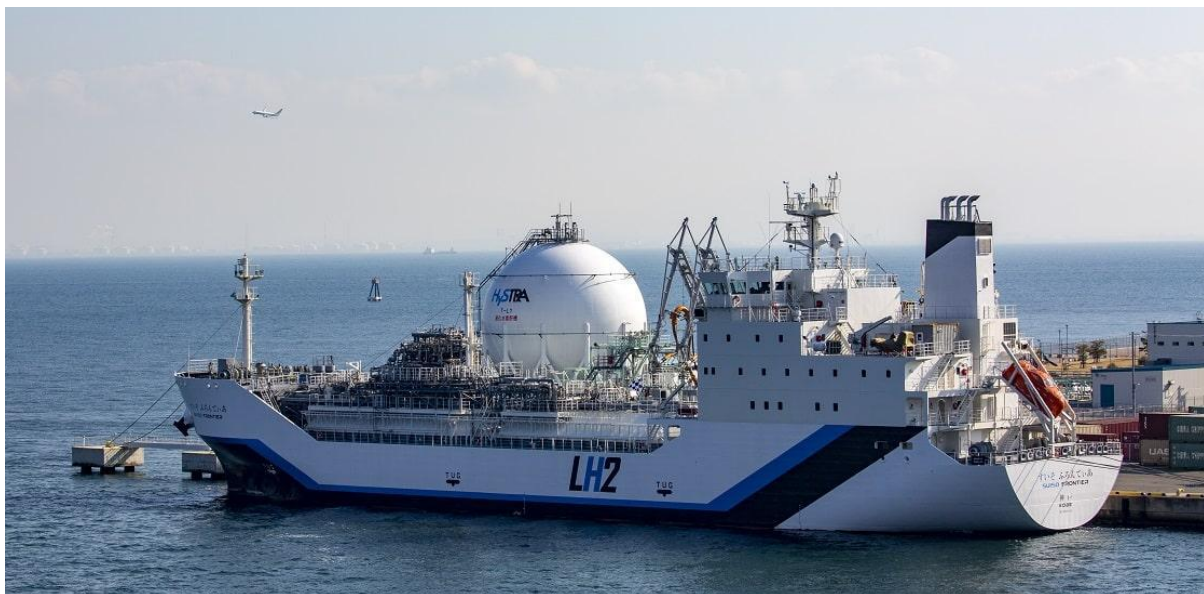
Figure 25: The world's first liquid hydrogen carrier Suiso Frontier berthed at a hydrogen terminal in Port of Kobe, Japan. Image: HySTRA.
