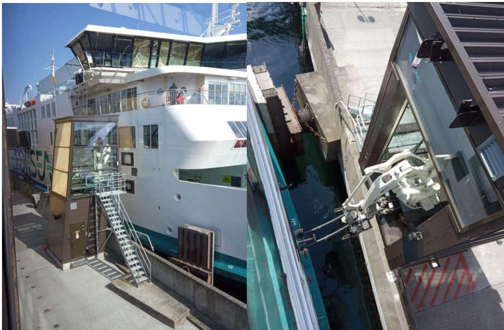
Figure 5: Shoreside 10.5 MW charging connection for Aurora af Helsingborg and Tycho Brahe passenger ferries (images: ZESTAs).
