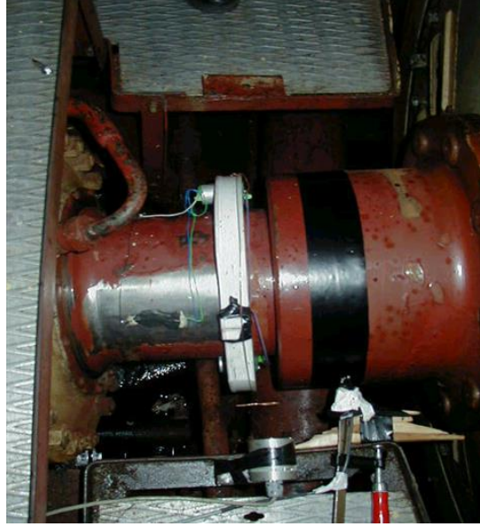
Figure 1 Strain gauges mounted on the propeller shaft
