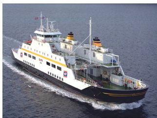
Glutra (IMO 9208461), the first 100% LNG-fueled ship 68)
