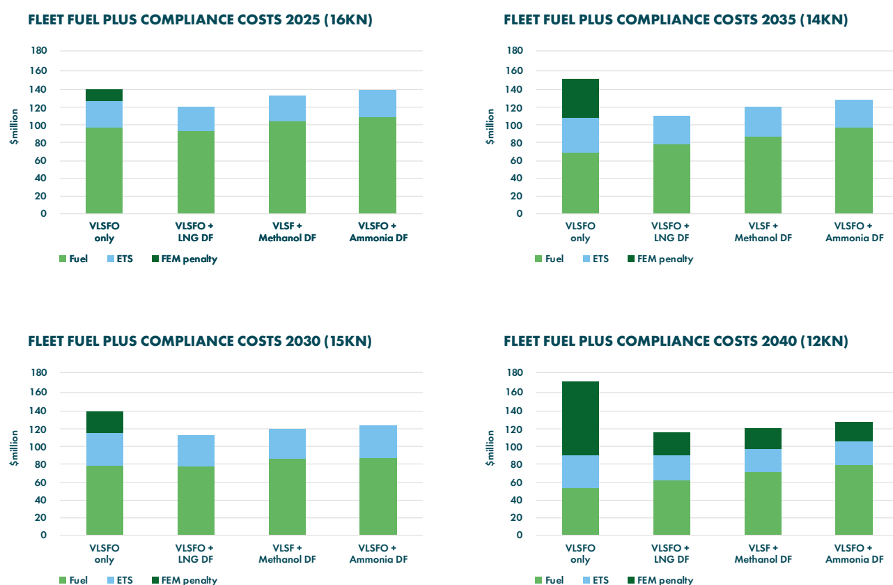
Figure 8: Scenario 1: Fleet cost breakdown by vessel speed
