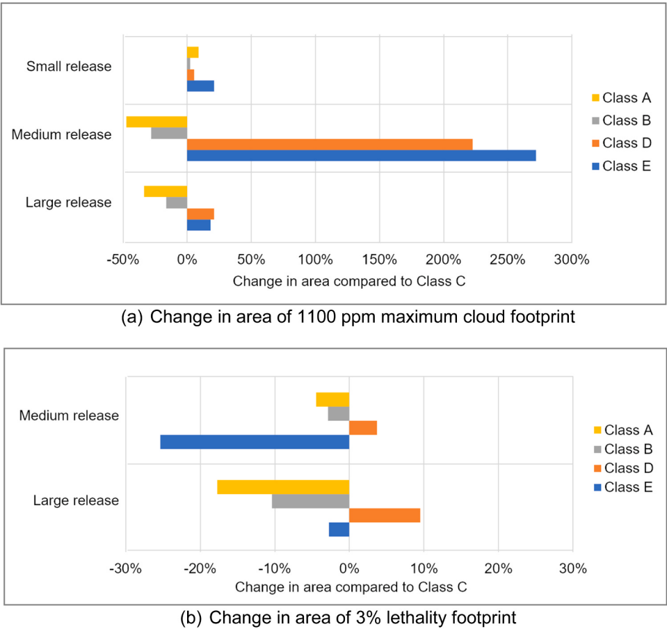
Fig. 10. Variations in 1100 ppm maximum cloud footprint and 3% lethality footprint compared to Class C Pasquil stability.
