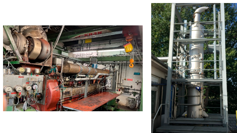
Figure 1. Measurement setup at Flensburg University of Applied Sciences: MaK Engine (left) and Scrubber (right).
