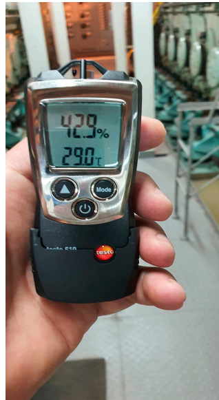
Figure 7. Humidity measuring instrument “Testo 610”, used for measurements on an LNG ship.
