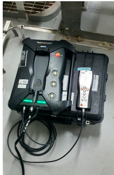
Figure 3. Exhaust gas analyzer “Testo 350 Maritime”, used for measurements on an LNG ship.
